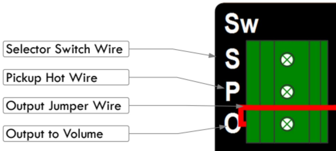
**Figure D: Switch Connector**
